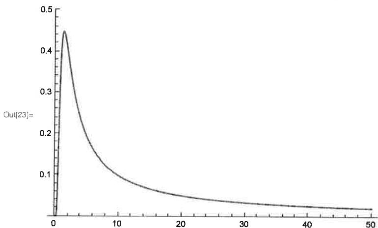
We realize that except for different units, and an additional factor of "T", Chi[T] and C[T] have identical forms. So X will still go to zero as T->0, and X will still go to 0 as T->∞ albeit not quite as fast as C will. Both of these are response functions, C is a response to added energy and X is a response to added magnetic field strength.
