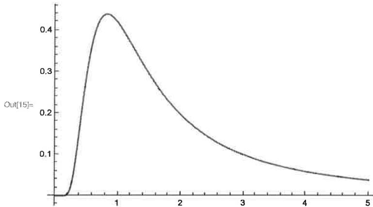
We see that C has a broad maximum, which is in the region of T's where M(T) is falling from the value of 1.0 (perfectly aligned spins) toward 0.0 (randomly aligned spins). In this region, the system is able to take on energy by flipping spins, so it is able to receive energy (from a bath ...) and this is reflected in a change in temperature.
